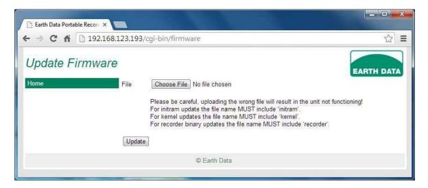
Choose the relevant file, using the indicated button. Note that in order to update the 'initram' the 'initram' file name will include 'initram', similarly kernel update will include 'kernel' and recorder binary update will include 'recorder' in the file names respectively.
